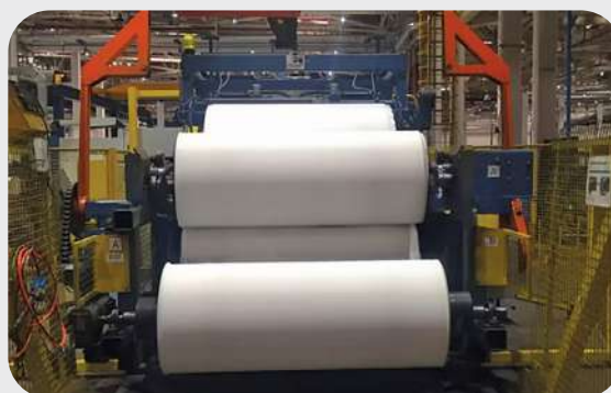
Tyre Lining - Rubber Calendaring Process
